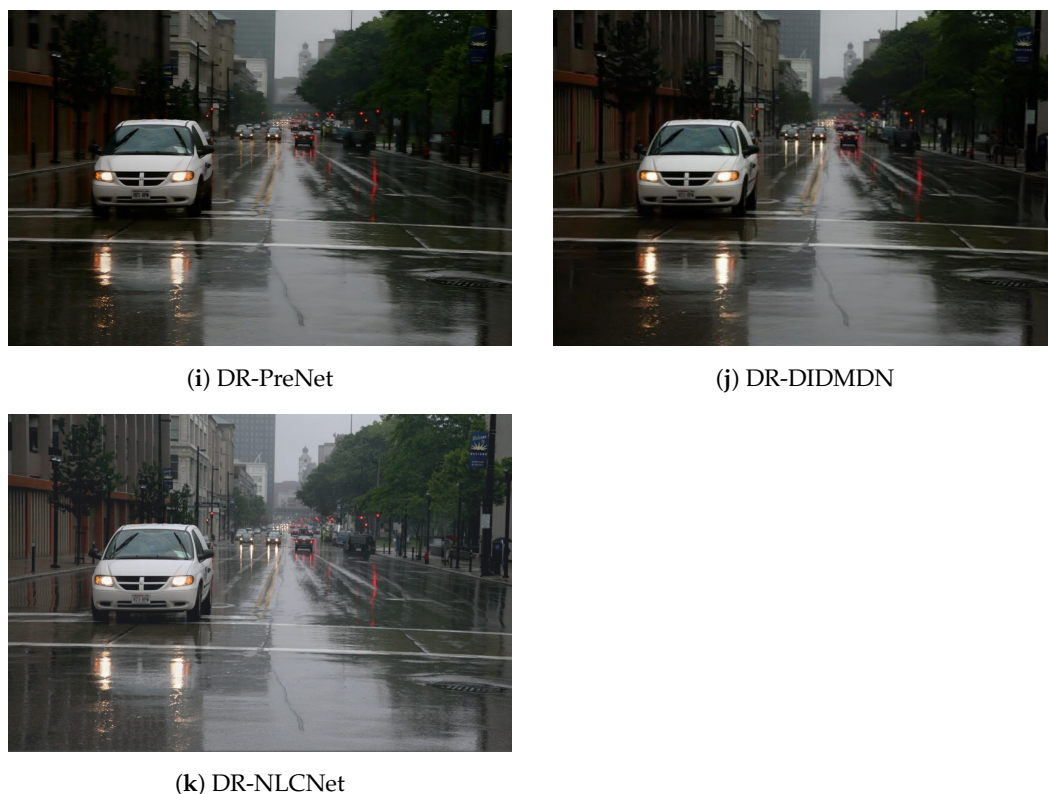
Figure 7. Deraining sample images. The best clarity in the top-right region (below the tree) is obtained using NLCNet. PromptIR, FDTANet, PRENet, and DIDMDN show a darker effect in that area.
